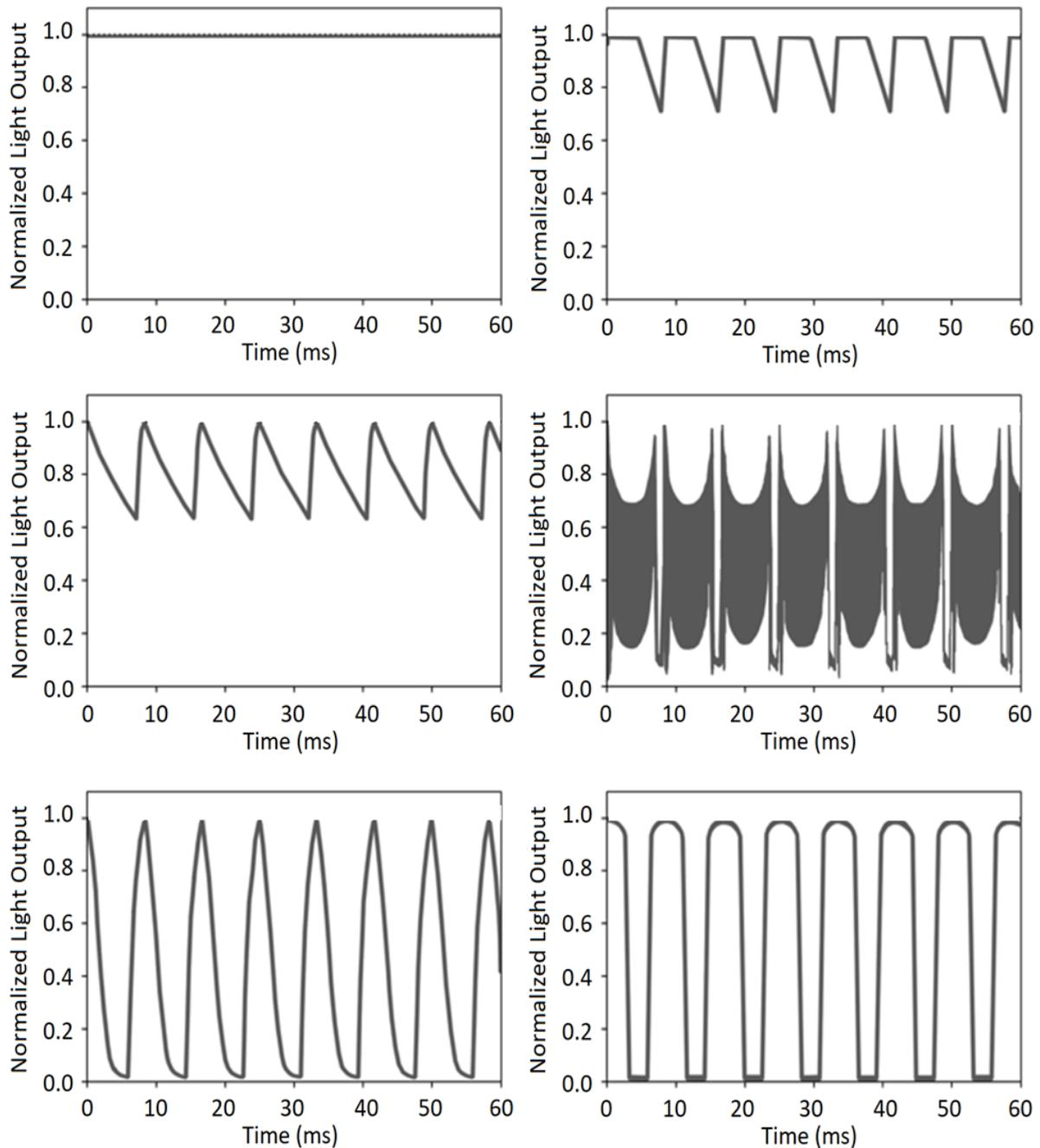
**Figure 2. TLM waveforms from a variety of LED systems, showing the wide variation. (Source PNNL).**
