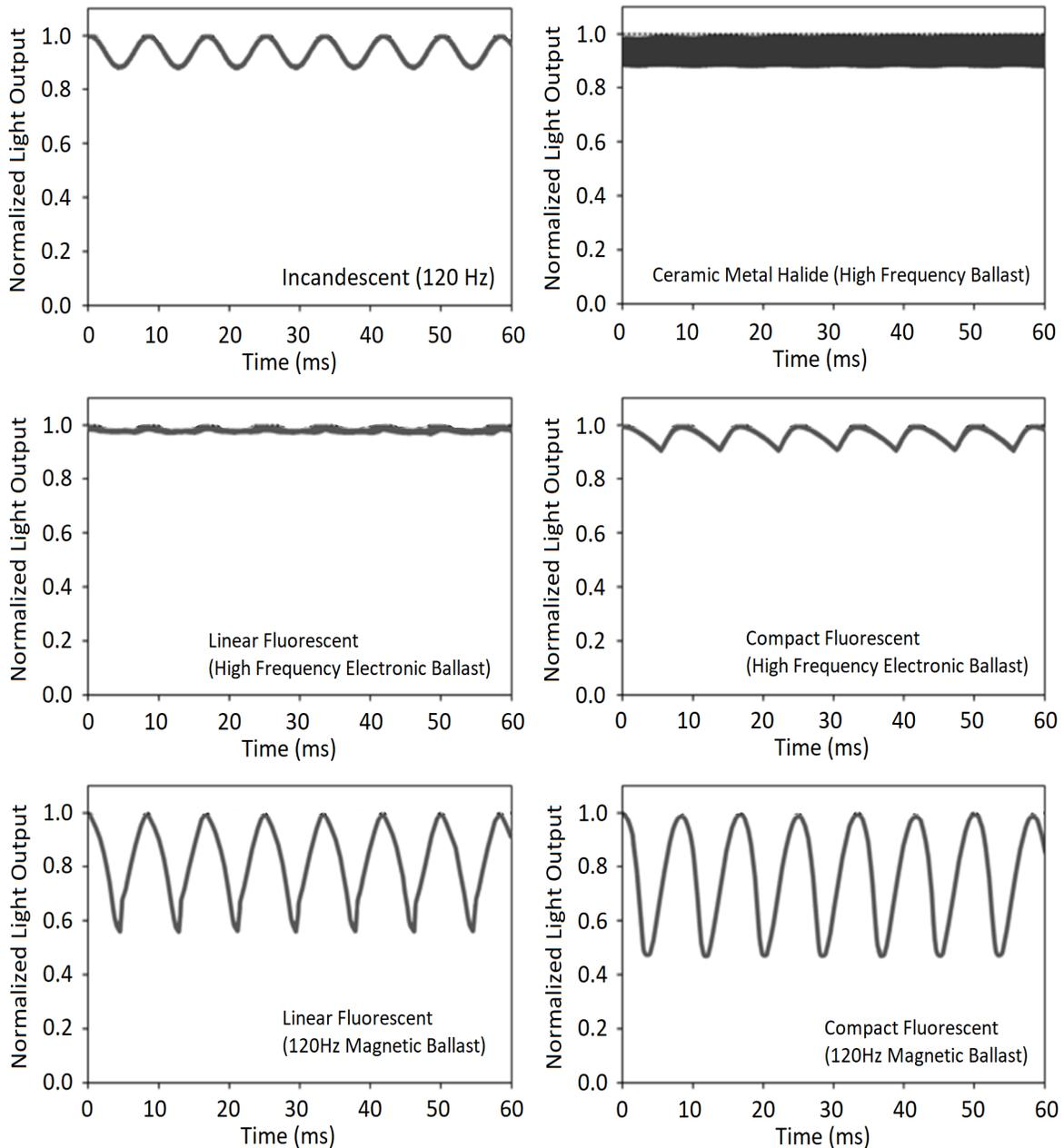
**Figure 1. TLM waveforms from a variety of conventional lamps and ballasts. (Source PNNL).**
