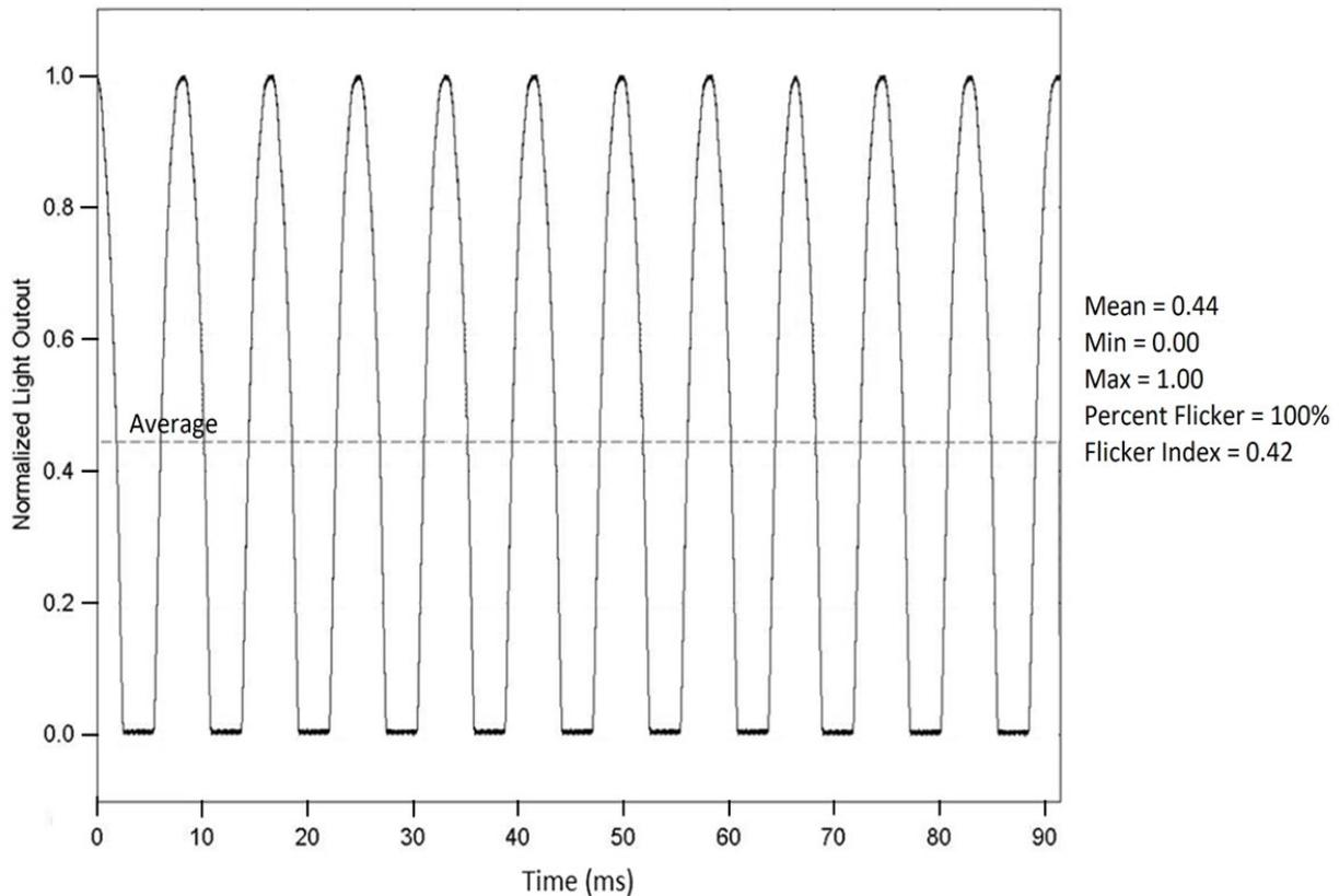
Figure 3. Waveform for an early AC-LED source, producing 120 Hz modulation. (Source: PNNL)
