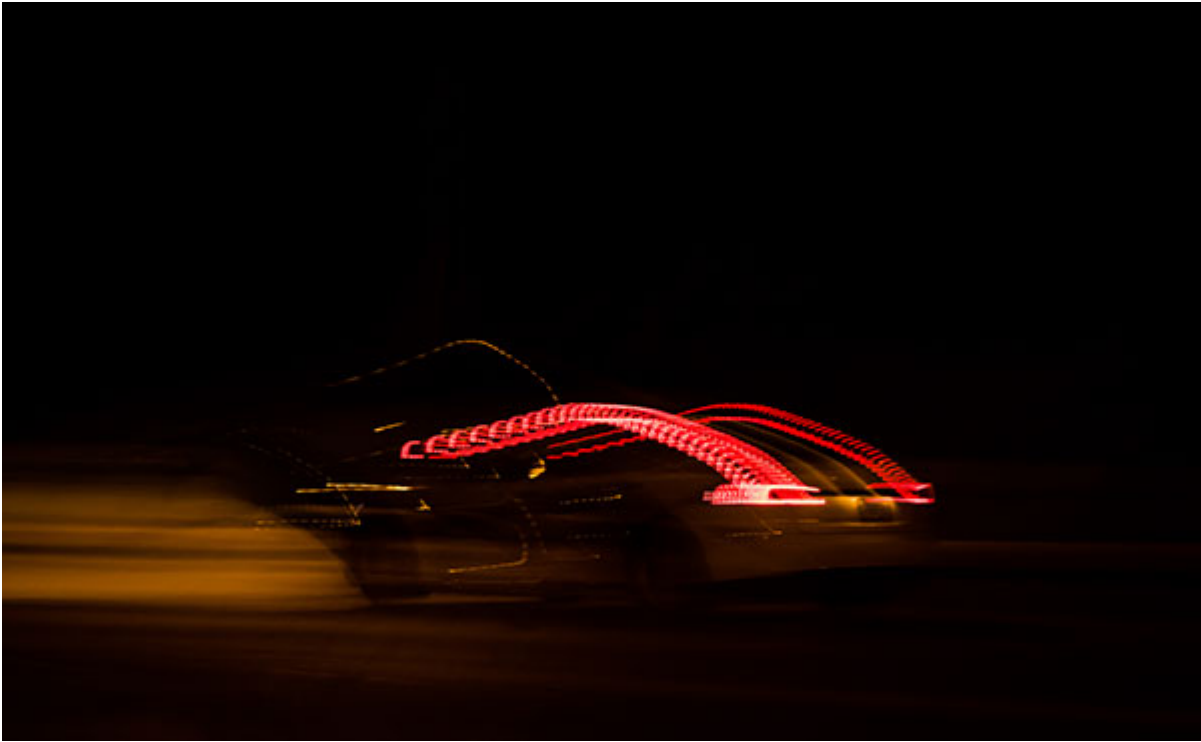
Figure 2. An example of a phantom array seen in taillights at night.
