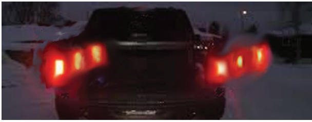
FIG 1 When a person's eyes move quickly from side to side, multiple images are observed in some LED car taillights.
