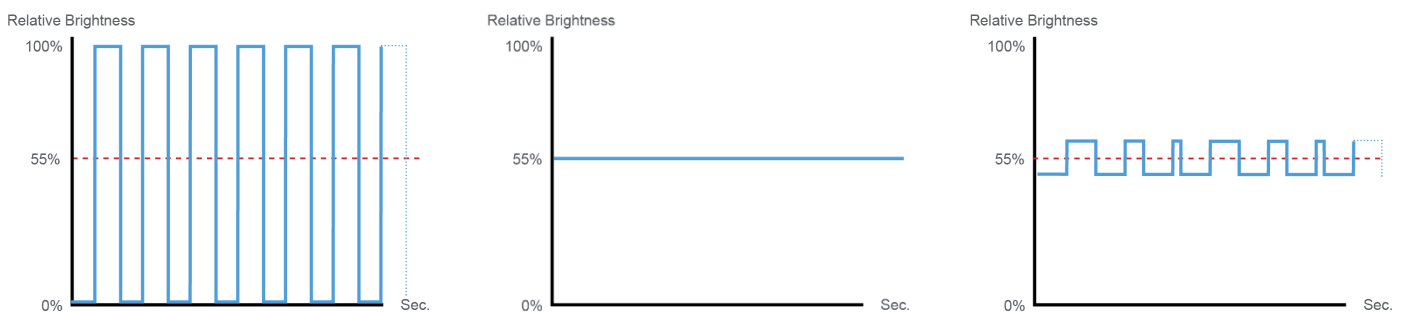
Figure 8 – LED dimming methods
