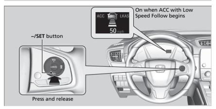
When driving at about 25 mph (40 km/h) or above: Take your foot off the pedal and press the –/SET button when you reach the desired speed. The moment you release the button, the set speed is fixed, and ACC with Low Speed Follow begins.
