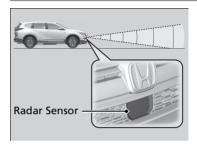
The radar sensor is in the front grille.
