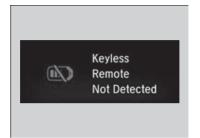
When the power mode is set to any mode other than OFF and you remove the smart entry remote from the vehicle and shut the door, an alarm will sound. If the alarm continues to sound, place the smart entry remote in another location.
