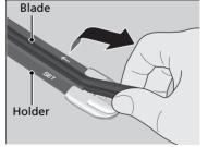
**6.** Pull the wiper blade in the opposite direction to slide it out of the holder.
