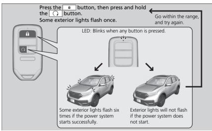
The power system is on for up to 10 minutes without you starting the vehicle. To extend the time for another 10 minutes during the first 10 minutes, press the
