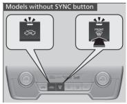
Pressing the 🕎 (windshield defroster) button turns the air conditioning system on and automatically switches the system to fresh air mode.
