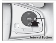
Press the 🖹 (Interval) button to change the ACC with Low Speed Follow followinginterval. Each time you press the button, the followinginterval (the interval behind a vehicle detected
