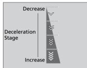
The default deceleration stage is  $\bigcirc$ . Each paddle selector operation makes a single stage deceleration change.
