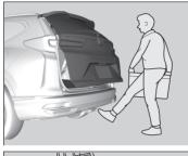
Use a forward and back kicking motion for about 1 second under the center of the rear bumper to open or close the power tailgate while carrying the smart entry remote.
