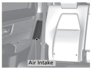
If the air intake is obstructed during vehicle operation, the High Voltage battery can become too hot. To protect the battery, the system may start to limit the battery's output and cause the power system and 12-volt battery charging system indicators to come on.
