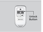
**To open:** Press the unlock button, and then within 10 seconds, press it again and keep it pressed. If the windows stop midway, repeat the procedure.
