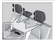
A passenger sitting in the rear seat should adjust the height of their head restraint to an appropriate position before the vehicle begins moving. **To raise the head restraint:** Pull it upward. **To lower the head restraint:** Push it down while pressing the release button.
