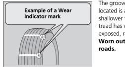
The groove where the wear indicator is located is about 1/16 inch (about 1.6 mm) shallower than elsewhere on the tire. If the tread has worn so that the indicator is exposed, replace the tire. **Worn out tires have poor traction on wet roads.**
