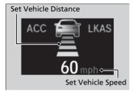
When ACC with Low Speed Follow starts operating, the vehicle icon, distance bars and set speed appear on the driver information interface.
