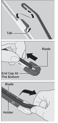
4. Press up on and hold the tab, then slide the holder off the wiper arm.
