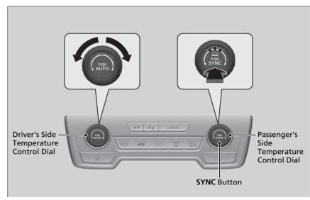
You can set the temperature synchronously for the driver's side and the passenger's side in synchronization mode.
