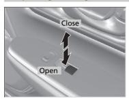
**To open:** Push the switch down. **To close:** Pull the switch up.
