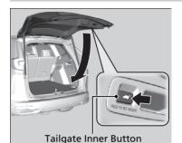
Press the tailgate inner button on the tailgate to close the power tailgate. ► The beeper sounds.
