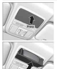
To open the sunglasses holder, press and release the indent. To close, press it again until it latches.
