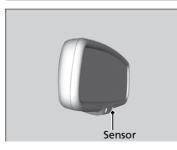
When you are driving after dark, the automatic dimming rearview mirror reduces the glare from headlights behind you. This feature is always active. Automatic Dimming Rearview Mirror\*
