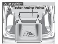
A tether anchor point is provided behind the rear outer seating position and in the ceiling for the rear center.
