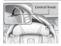
When the brightness of the meter will be reduced, you can use the brightness control knob to adjust instrument panel brightness. **Brighten:** Turn the knob to the right. **Dim:** Turn the knob to the left.
