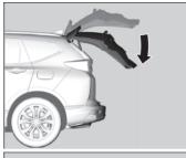
The extent to which the power tailgate automatically opens can be programmed.
