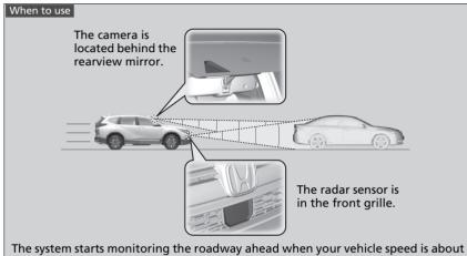
The system starts monitoring the roadway ahead when your vehicle speed is abou 3 mph (5 km/h) and there is a vehicle in front of you.
