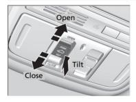
■ Automatic operation To open: Pull the switch back firmly. To close: Push the switch forward firmly.
