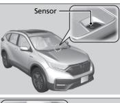
The automatic climate control system is equipped with sensors. Do not cover or spill any liquid on them.
