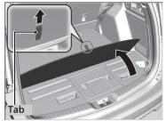
**1.** Using the tab, fold back the cargo area floor lid.
