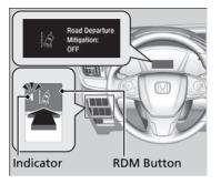
Press the RDM button to turn the system on and off.
