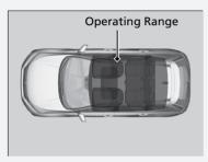
The power system may also start if the smart entry remote is close to the door or window, even if it is outside the vehicle.
