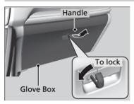
Pull the handle to open the glove box. You can lock the glove box with the built-in key.
