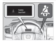
The seat belt system includes an indicator on the instrument panel to remind the driver or a front passenger or both to fasten their seat belts.
