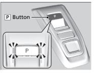
The shift position changes to  $\[P\]$  when you press the  $\[P\]$  button while the vehicle is parked with the power mode in ON. The indicators on the sides of the  $\[P\]$  button come on.
