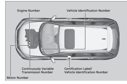
Vehicle Identification Number (VIN), Engine Number, Motor Number, and Transmission Number
