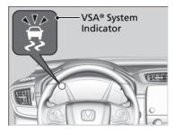
When VSA® activates, you may notice that the engine and motor do not respond to the accelerator. You may also notice some noise from the hydraulic brake system. You will also see the indicator blink. Wehicle Stability Assist<sup>™</sup> (VSA<sup>®</sup>), aka Electronic Stability Control (ESC), System
