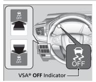
This button is on the driver side control panel. To partially disable VSA<sup>®</sup> functionality/ features, press and hold it until you hear a beep.
