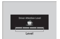
When the (display/information) button is pressed, bars in the Driver Information Interface light up in white to indicate the degree of the driver's attention.
