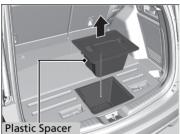
**2.** Remove the plastic spacer from the cargo area.
