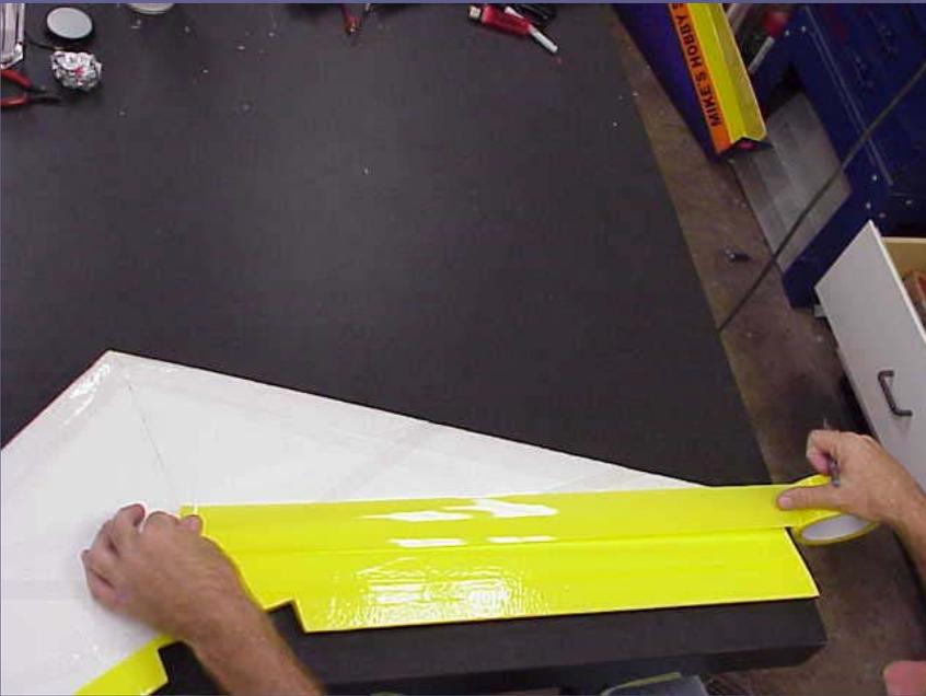
● Make sure to trim the tape with a slight curve near the leading edge at the tip to allow the tape to lay flat on the tip.
