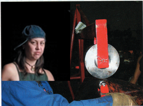
Lynn Bryant taking hammer marks out of the copper egg shell on the English wheel. Lynn and her team were also responsible for the construction and design of the Egg. Lynn told me that she's real good at making wagon wheels and elbow macaroni after bending all of the steel tubing used in the egg's framework.
