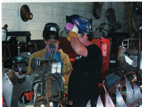
Rebecca "Hot Metal" Anders and Charlie Gadeken weld yet another stainless steel vertebrae together. The respirators are worn to protect the Girls from the dust, gasses, and nasty chromium by-products that are produced when grinding or welding stainless steel. It gives you a bad headache. The manufacturer painted them pink for some reason. Although, hot pink is the official color of any tool or part claimed (often by convenience) by the Girls at the Box Shop.
