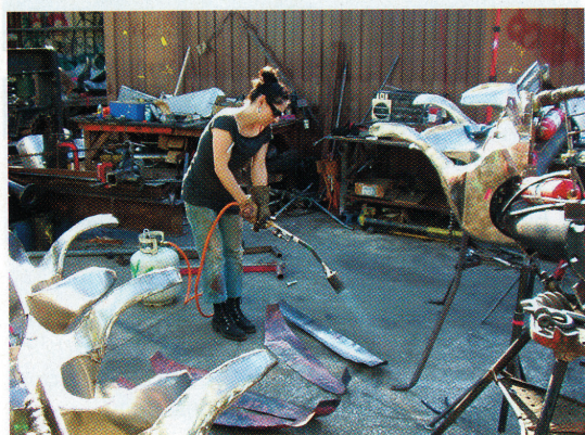
Annealing copper with a big torch to make it soft for shaping. Once shaped, the metal is then hammered until it hardens to hold its shape and then it is soldered together to make larger pieces.
